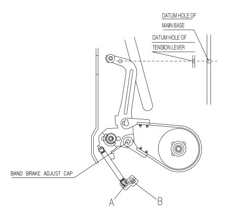
Fig.4-7 TENSION POLE POSITION ADJUSTMENT
